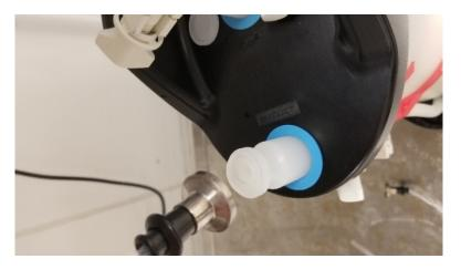
Figure 18. Disconnect small column tubing ends for connection to outlet port
