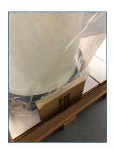
Attach reusable corrugated ramp to crate base using reinforced Velcro strips.
