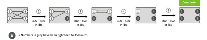
Figure 1B. 2-Bolt numbered torque sequence | Appropriate for 0.1 m<sup>2</sup> cassettes
