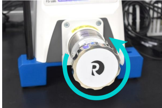
Figure 13. Loosen the pressure plate by rotating counterclockwise.
