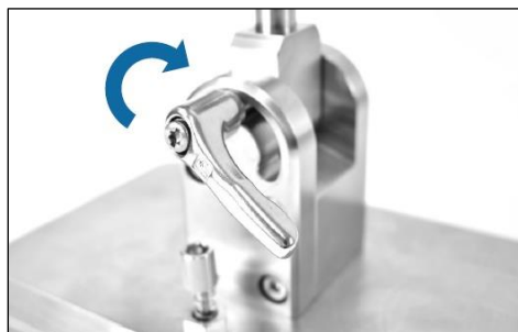
Figure 24. Tighten Mounting Post Clamp Handle
