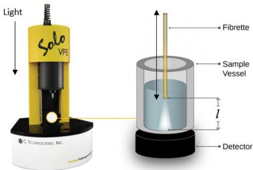
Figure 3: Schematic principle of variable pathlength of SoloVPE method [12]
