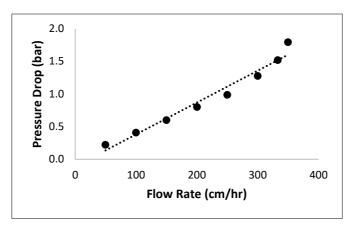
Pressure drop was measured with increasing linear flow rate from 50 - 400 cm/hr (Figure 1). NGL COVID-19 Spike Protein AR 2.0 Resin was packed in an OPUS<sup>®</sup> 45R Column (45 cm D x 20 cm L). Compression factor: 1.2; mobile phase: 0.1 M NaCl.
